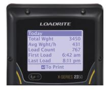
In-cab metrics feedback to the operator during the shift
