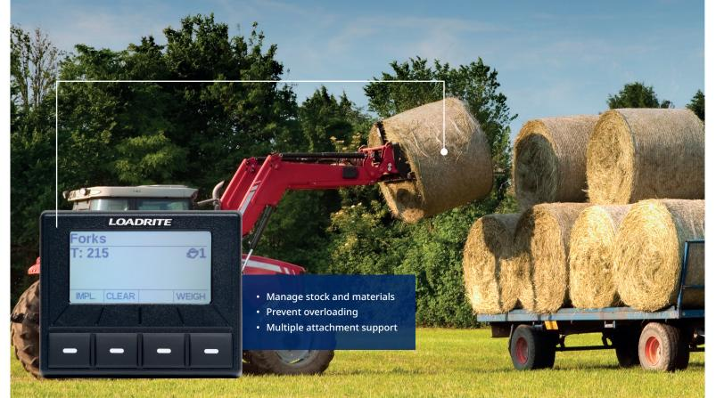
Cost-effective, compact, all-weather measurement of construction materials and farm feeds. The Loadrite<sup>®</sup> S1100 is an on board scale that helps the operator to accurately weigh every lift, track loading totals, prevent overloading and effectively manage stock. So you can improve safety and profitability through increased efficiency and accuracy.
